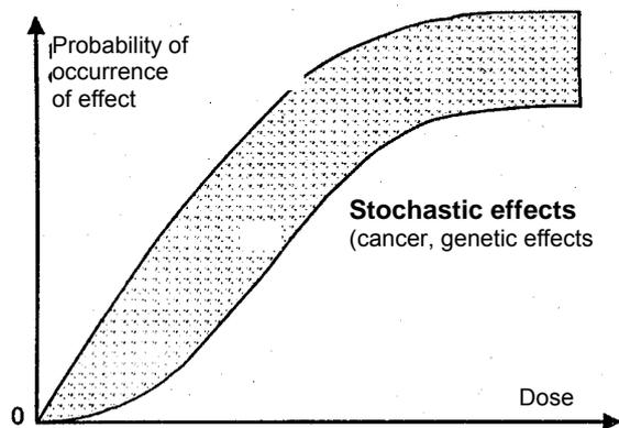
Fig. 3.1: Probability of occurrence of a stochastic effect as a function of the dose /SSK 96/<sup>2</sup>
